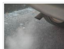
In urban areas, most nanoparticles come from diesel engines or cars with defective or cold catalytic converters
